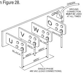
Figure 28. UVWO Terminal Lugs 1Ø-480V Connections
